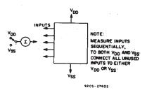
Fig. 9 - Input-current test circuit.
