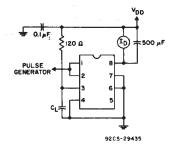
Fig. 7 — Power-dissipation test circuit for CD401078E.
