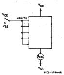
Fig.8 - Quiescent-device current test circuit.
